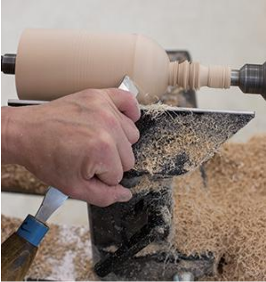
Cutting the right side of a bead with a skew.
