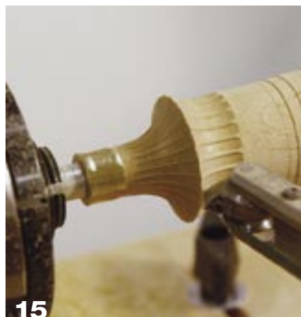
15 With a belt-driven fly cutter, make your ornamental cuts at the headstock end.
