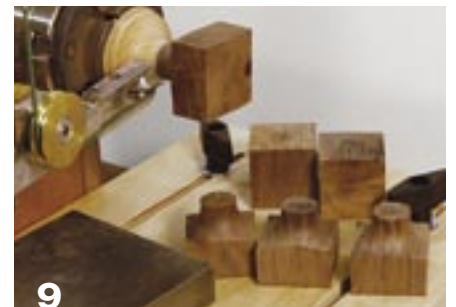
9 Turn down the shoulder of each knob. A belt-driven cutting frame, left , does the work.
