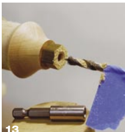
13 Drill the handle to the depth of the tool-holder shank; most shanks are about 1".
