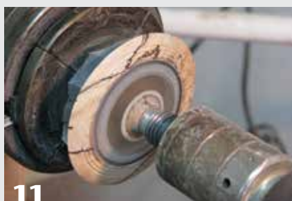
11 Turn away the tenon and bottom layer of wood. With the tailstock in place, a nub will remain that cannot be turned away. Here, I left a large nub, but it can be much smaller if you use a cone on the live center.
