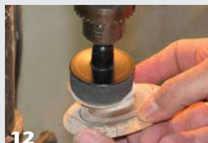
12 Sand away the nub using a sanding attachment chucked in a drill press.
