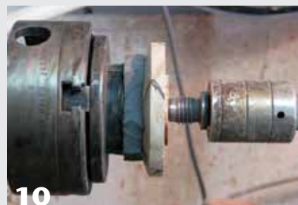
10 An alternative to the vacuum chuck: press the workpiece with the tailstock live center against a soft pad held in a chuck.
