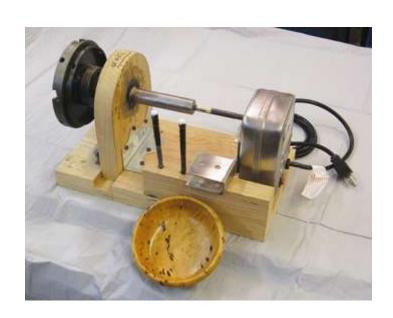
Drill into the end of the 1" (25mm) bolt so that the .375" (10mm) bolt sets .75" (19mm) into it. Drill and tap the inside of the 1" (25mm) bolt to hold the .375" (10mm) bolt with a setscrew. Loosen the setscrew when applying finish. The 1" (25mm) nut, which is also drilled and tapped, serves as a stop for the chuck.
