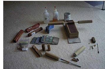
Using the hand mandrel as shown to shape the the blank on the sanding block( 80 grit). When shaping is down to the brass, the brass is removed leaving the slimline bushings. Next using 150 to 600 grit, it is hand sanded from handle to handle removing scratches caused by the 80 grit. The blank will be down to the bushings. Now micro mesh can be used for a great shine.
