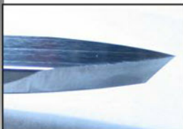
Photo 1: Side Profile. 1" wide x 0.25" thick, Bevel angle ~45 degrees
